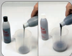
1. 1. Pour the 2 components in a 1:1 ratio in the measuring beaker
