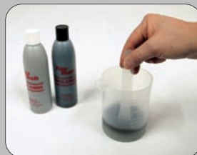
2. Mix in the beaker for 30 seconds max
